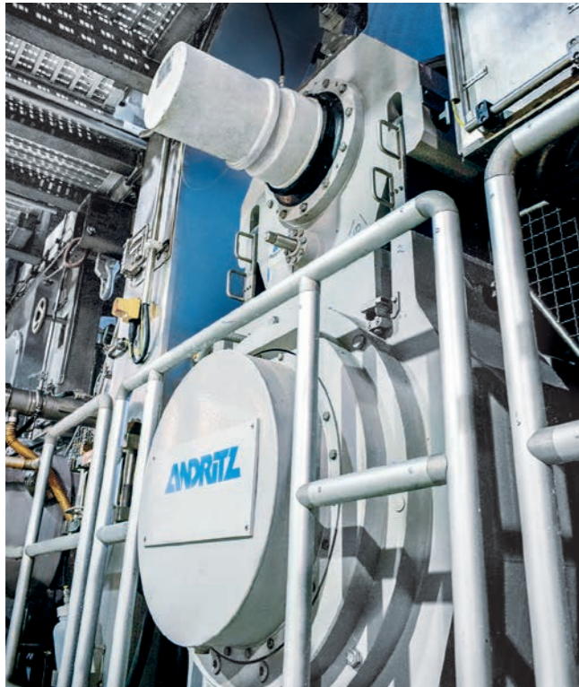
The ANDRITZ PrimePress X shoe press is a very low-maintenance design which gives the Iggesund Workington mill the required bulk and dryness for its premium board products.
