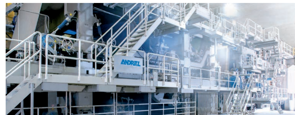
From a seven-ply suction former to a two-ply machine with press section.
