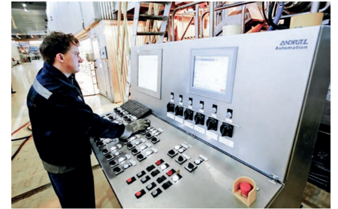
ANDRITZ Automation integrated existing and new features into its DCS and QCS systems.
