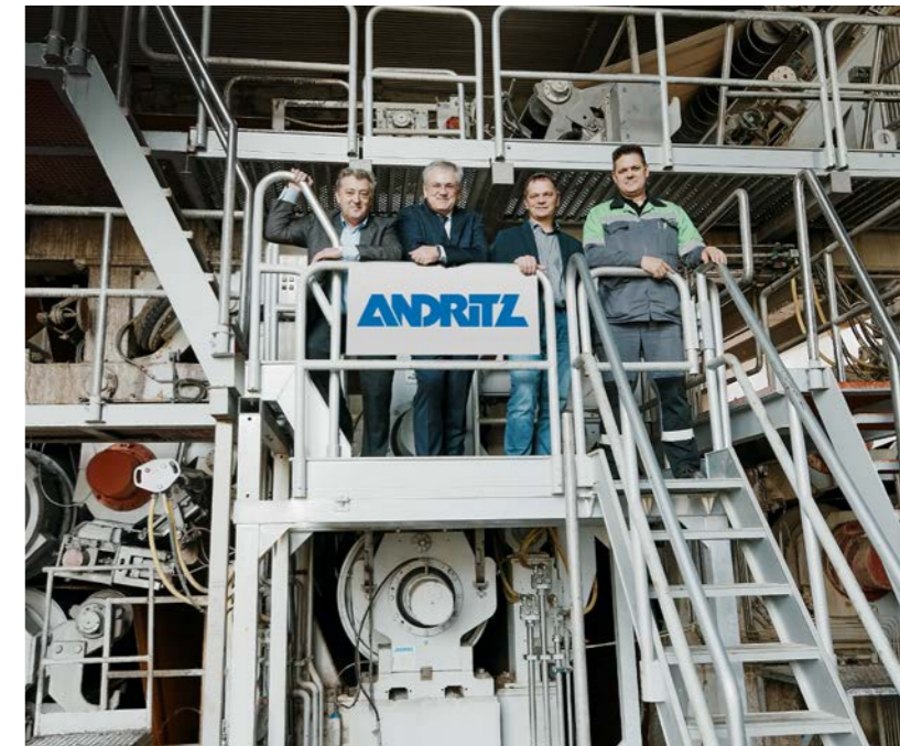
The upgraded press section on BM1 has a new geometry and increased capacity, with a new ANDRITZ PrimePress X shoe press in the original second position. (left to right) Aleksandr Yakovina, Georg-Michael Sautter, Aleksandr Kravchenko, and Vitaly Solovyov
