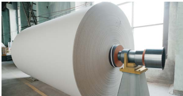
BM1 produces white-top liner and white-lined chipboard in a basis-weight range of 125-420 gsm.
