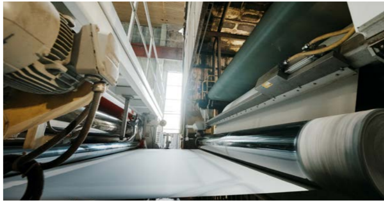
The upgraded calender section provides a consistent CD caliper profile, bulk control, and excellent surface finish.
