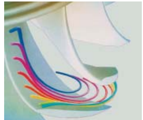
Computer generated streamlines through a Compact Francis Turbine runner
