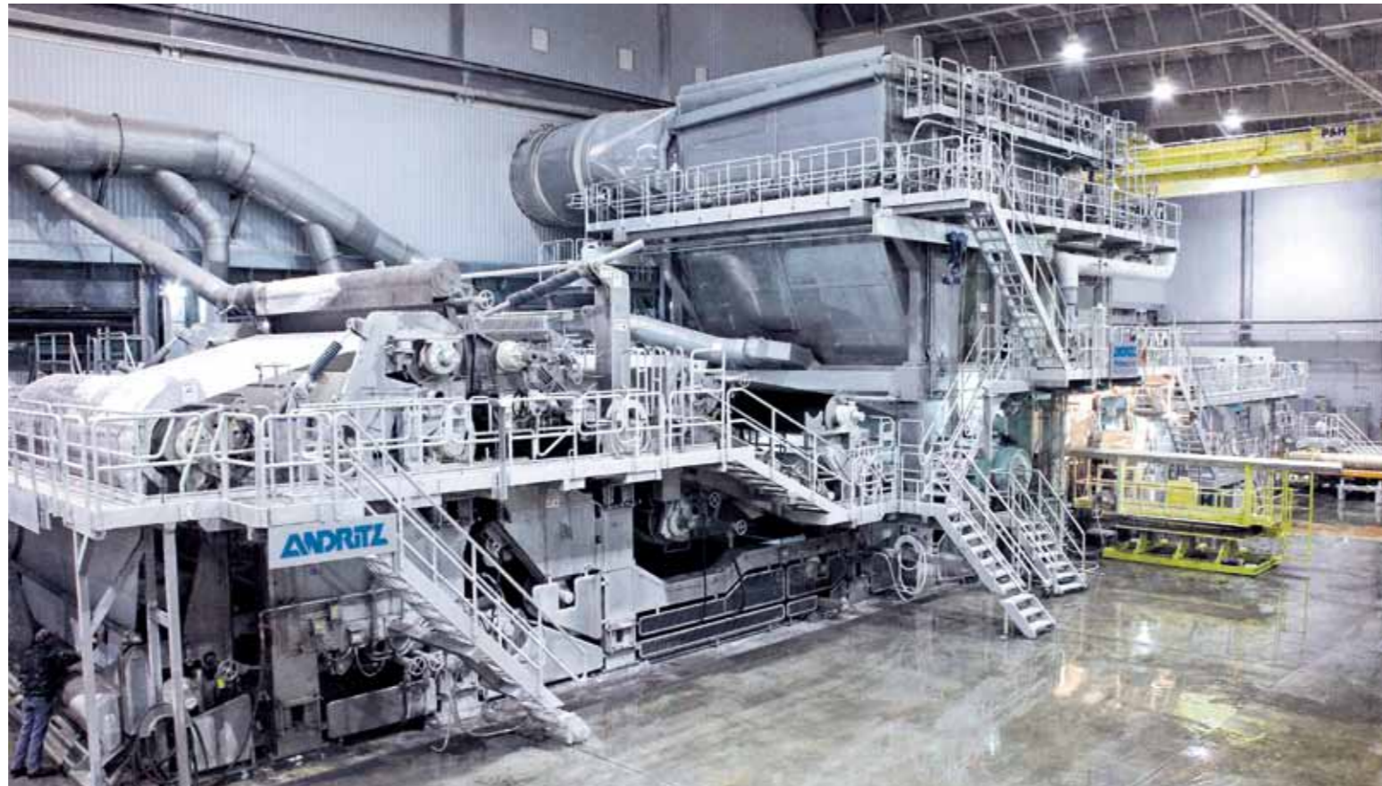
▲ "With the PrimeLine CrescentFormer, you get a very nice, filled-in sheet for lightweight grades," Jim Haeffele says. Shown above is the new PM 14 – a 5.5 m wide, 2000 m/min ANDRITZ tissue machine.
