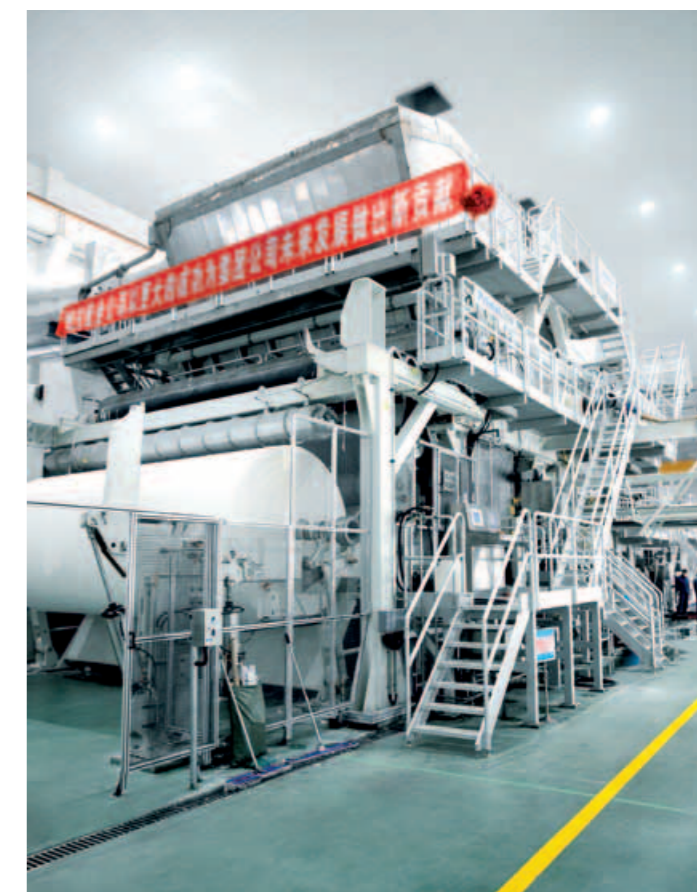
ANDRITZ delivered the production line – from stock preparation to the reel – turnkey. Parent rolls from the PrimeLine machine are converted into tissue products at the mill site. ▶
