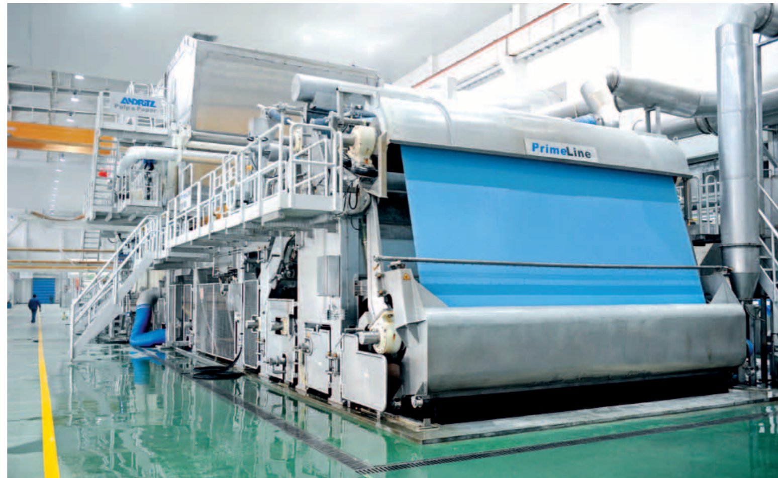
The PrimeLine™ W8 CrescentFormer machine at Hupo Paper. The 5.6 m wide machine has a PrimeFlow two-layer headbox and a PrimeProFiler F dilution control system. ▼
