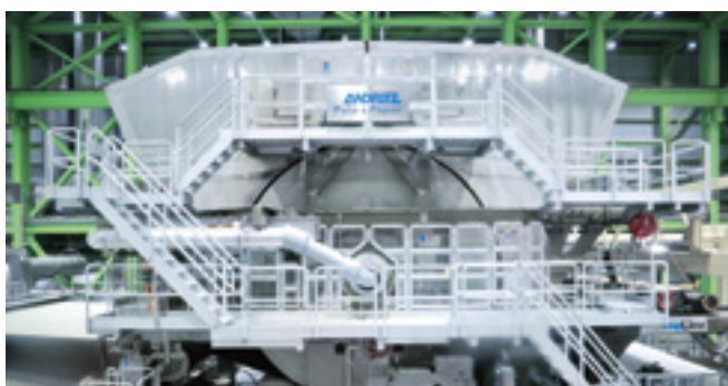
◀ St. Croix specified a large Steel Yankee (18-foot diameter) for both machines. TM1 started up in March and TM2 in July 2016.
