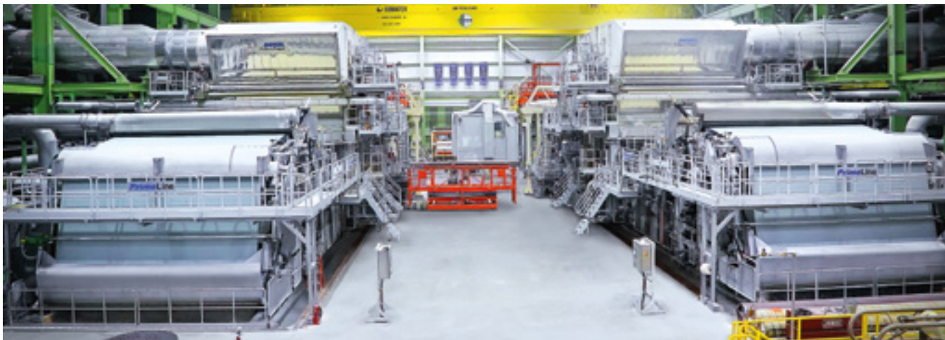
▲ Mirror-image PrimeLine tissue machines. Design speed is 2,000 m/min. Width 5.6 m. Capacity 126,000 t/a combined.
