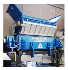
The Universal-Shredder ADuro U-3000X is a single-shaft shredder with electric drive & hydraulic driven pusher. The innovative CoverCross knife system cuts material to the required particle size in one step.
