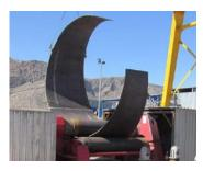
Ilisu, Turkey 2010; 1,224 MW Penstocks and gates Head / Length: 125.8 m / 267.5 m Diameter: 11 - 5.1 m Total weight: 12,000 tons
