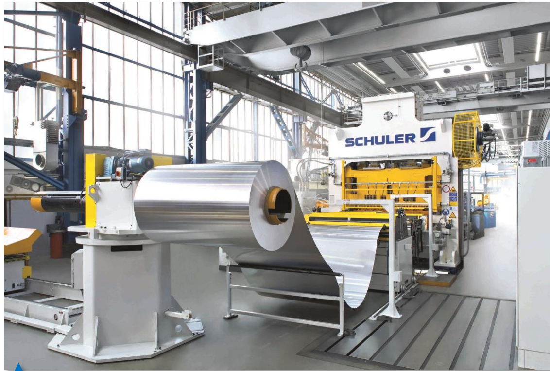
Cupping press, designed for production of 3,000 cans per minute
