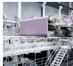
PrimeForm HB Hybrid former for excellent formation with optimal dewatering
