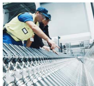
PrimeFlow SW Headbox with lamella technology and consistency profiling system
