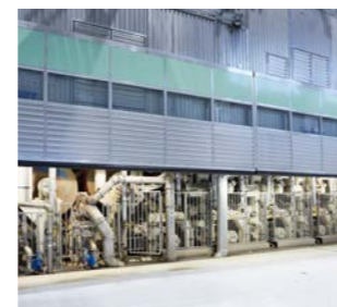
PrimeDry Pre-dryer section with double-tier drying group, web stabilizers, and steel cylinders
