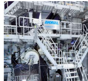
PrimePress Tri X Shoe press configuration and transfer belt. Developed together with Zellstoff Pöls AG
