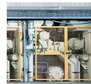
PrimeDry After-dryer section with double-tier drying group, web stabilizers, and steel cylinders
