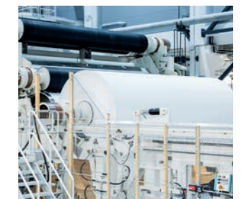
PrimeReel Fully automated turn-up process for diameters up to 3,000 mm
