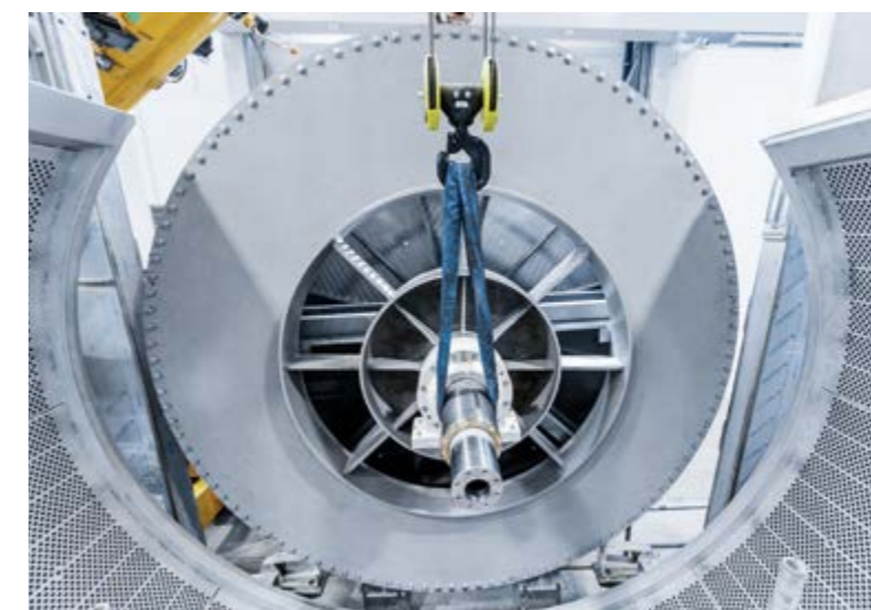
TAD-drum installation at the ANDRITZ tissue pilot plant
