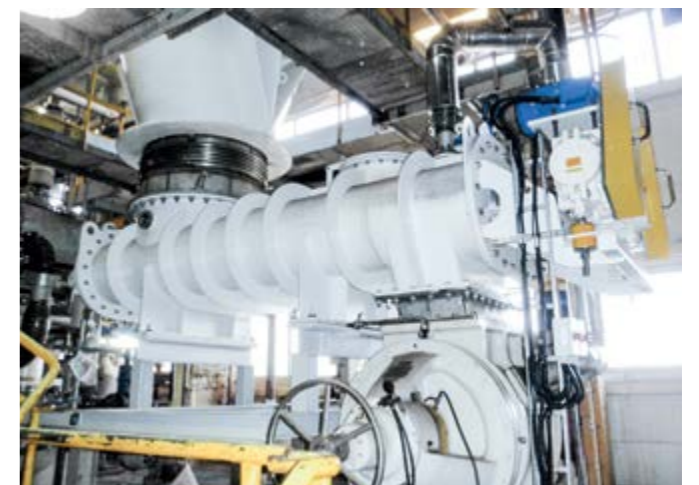
Diamondback™ chip bin bottom and chip metering screw provide uniform chip flow.
