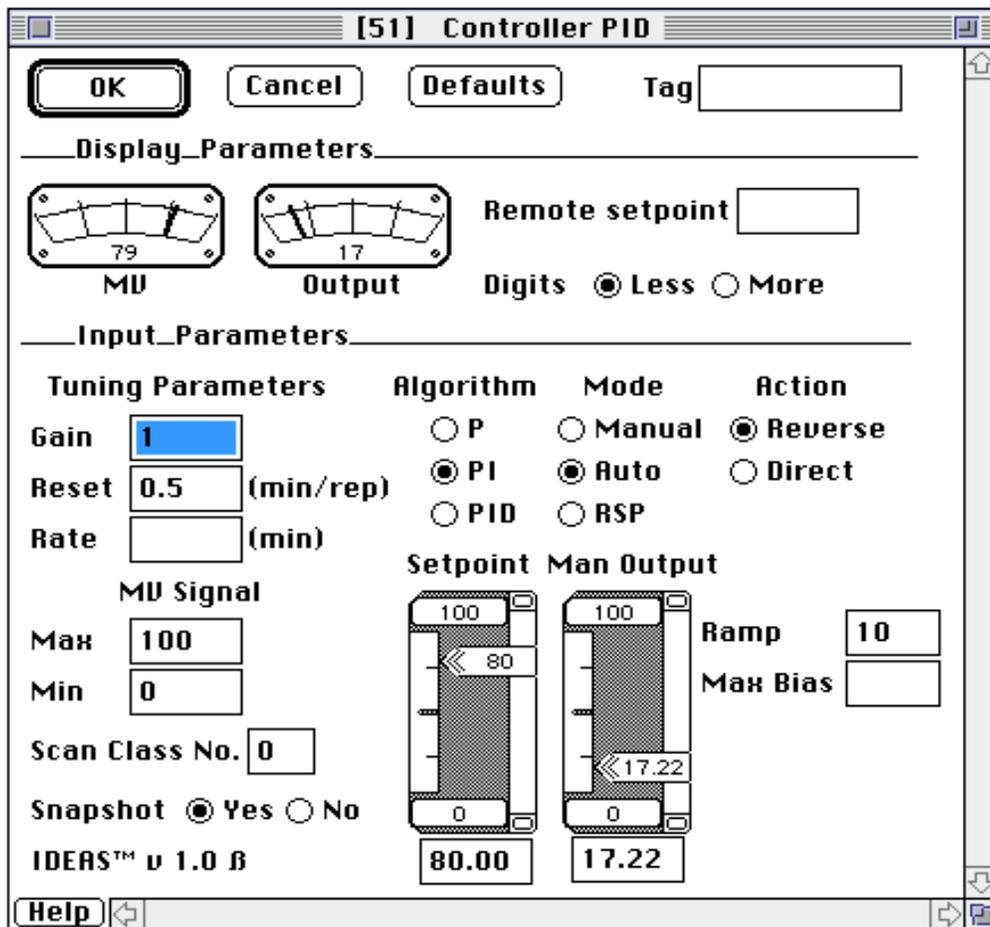
FIGURE 2. An IDEAS™ Dialog Box for a PID Controller
