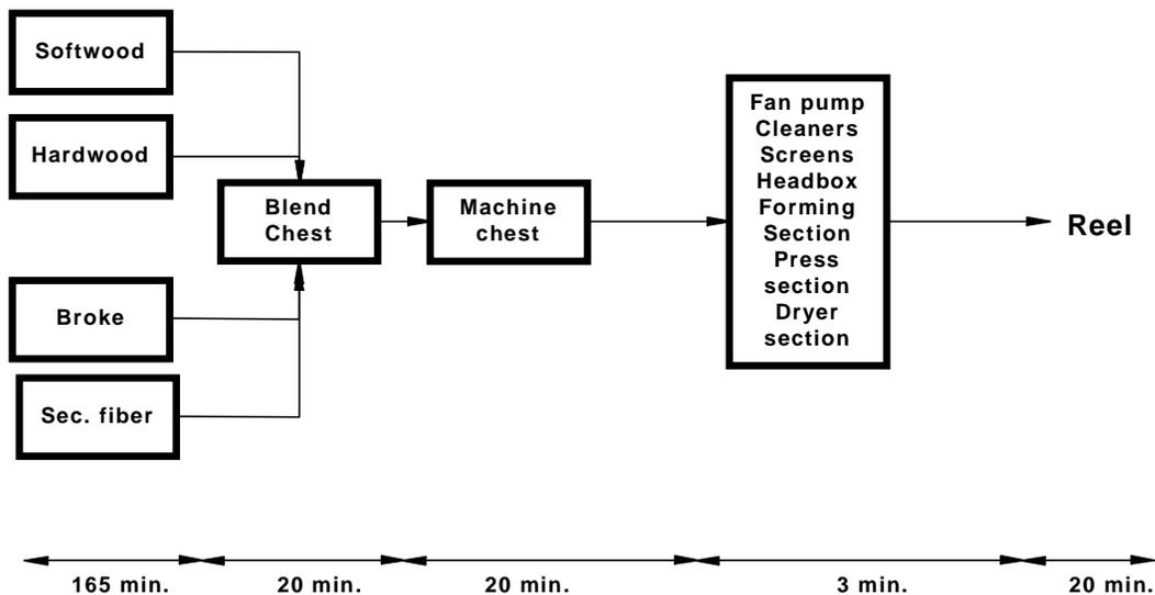
**Figure 1. Typical mean chest residence times throughout a papermaking system**
