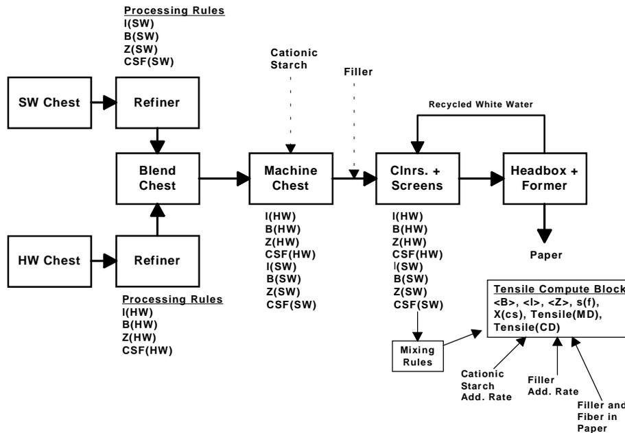
**Figure 5. Processing and mixing rules and other non-mass balance calculations required in the tensile simulation.**
