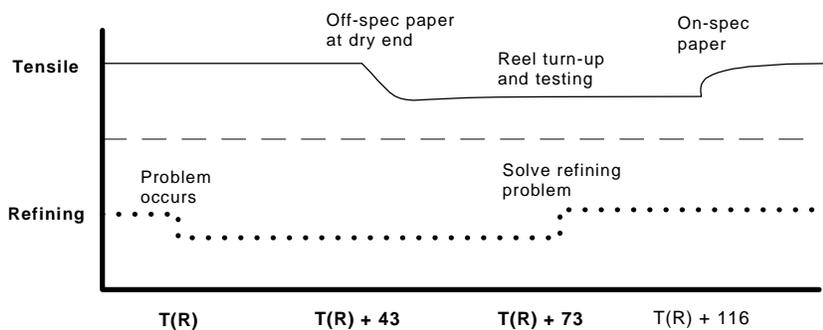
**Figure 3. Schematic illustration of off-quality paper production in the absence of a predictive model or on-line sensor. A total of 73 minutes of off-quality paper would be produced. It is assumed that the refining problem gets solved as soon as it is discovered.**
