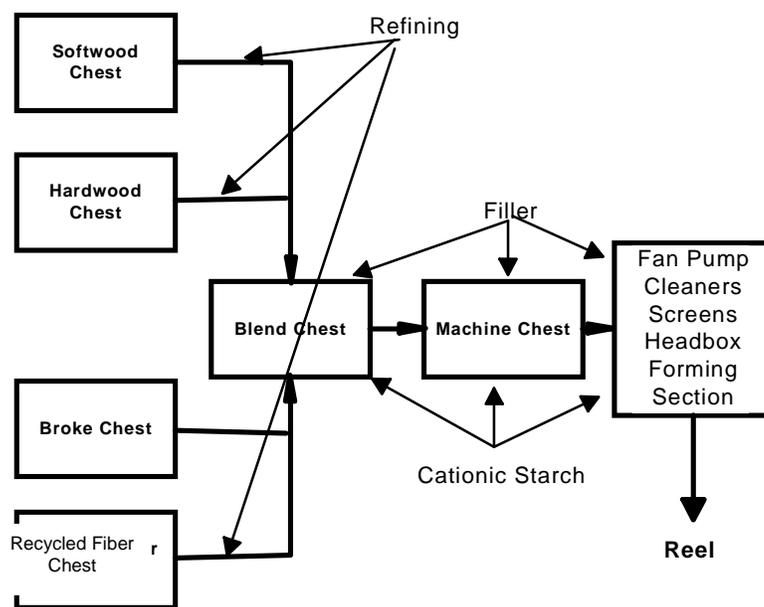
**Figure 2. Paper machine schematic diagram illustrating chemical additive addition points.**
