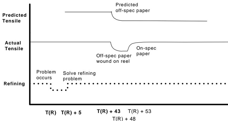
**Figure 4. Schematic illustration of off-quality paper production in the presence of a predictive model. A total of 5 minutes of off-quality paper would be produced. It is assumed that the predictive calculation occurs much faster than real-time. It is further assumed that the refining problem gets solved as soon as it is discovered.**
