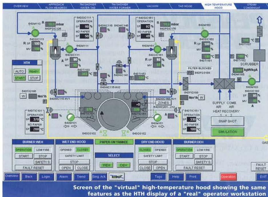
Screen of the "virtual" high-temperature hood showing the same features as the HTH display of a "real" operator workstation
