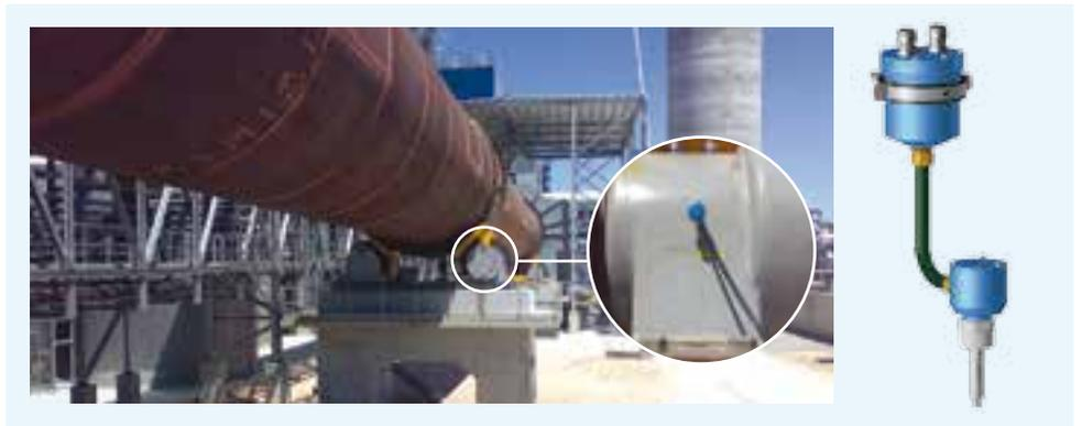
▲ The above photo shows the location of the ACU-230 sensor installed on a lime kiln carrying roller friction bearing. The sensor features a separate sensor head and electronics in separate aluminium enclosure, ideal for applications with high temperature at the monitoring area.
