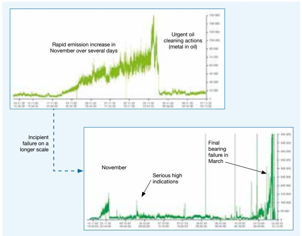
▲ Figure 1: Indications of incipient bearing failure and final breakdown as detected by Digester ACD
