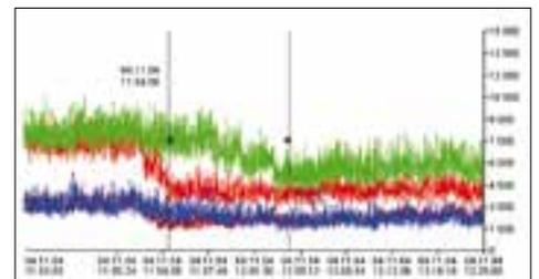
▲ Figure 5: Emission value change during seal bar adjustment
