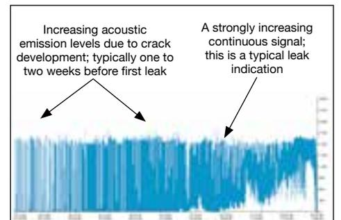
▲ Figure 4: Crack formation and leak on economizer as detected by Recovery Boiler ACD
