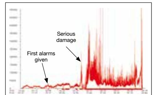
▲ Development of serious carrying roller bearing fault over a long period
