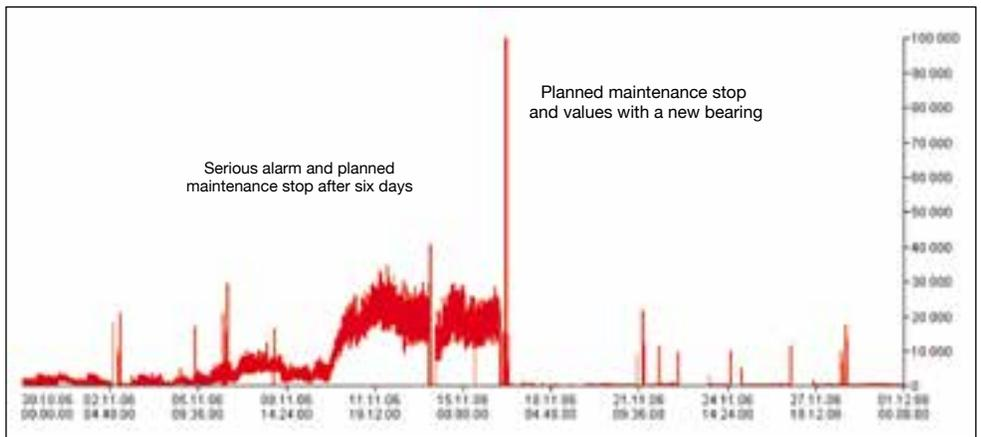
▲ Figure 7: Detailed view of the trend, showing serious fault development in roller bearing as detected by Pulp Dryer ACD
