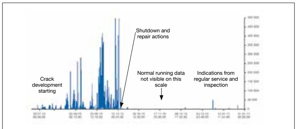
▲ Figure 2: Crack formation on a digester outlet device as detected by Digester ACD
