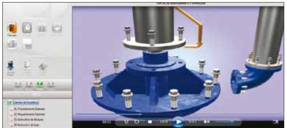
▲ Screen capture showing sequential disassembly operation 3D presentation in operator's native language
