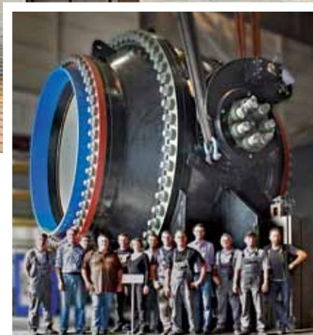
▲ Spherical valve for HPP Herdecke: completion of tightness testing after service
