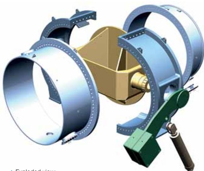
▲ Exploded view: main components of butterfly valve
