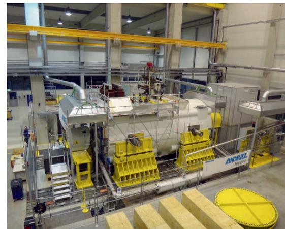
Hydrogen-cooled turbogenerator in test field
