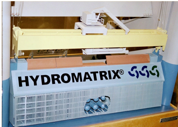
Figure 1: Upstream view on a HYDROMATRIX ® -Module /1/
