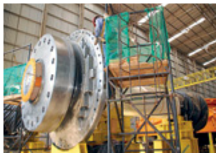
▼ Generator bearings for HPP Santo Antônio
