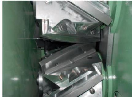
▲ Knife heads of edge scrap shear behind side trimmer
