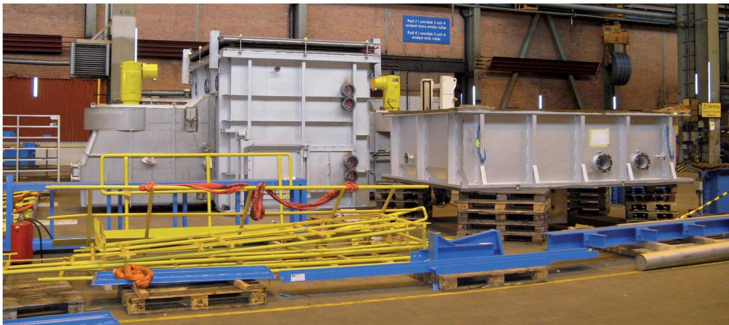
▲ Preassembly of equipment before erection: design and manufacturing are done for shortest maintenance stops
