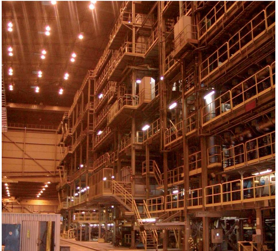
Elevation of the furnace: general view with soaking, jet cooling and re-heating ▲
