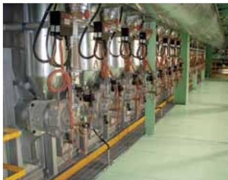
▲ Radiant tube furnace equipped with latest technology burners
