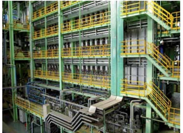
▲ The continuous galvanizing line (CGL) n°1 of TIANJIN ANSTEEL TIAN TIE in Tianjin started operation in June 2009. The All Radiant Tube (ART) furnace of this CGL has been designed and built by ANDRITZ Selas and allows the customer a high degree of flexibility due to its special design features.
