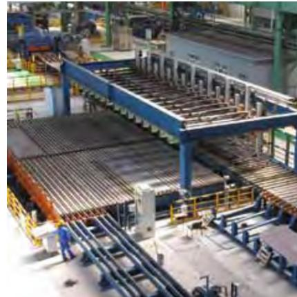
▲ Portal stacker for steel plates of dimensions up to 18 x 16,000 mm
