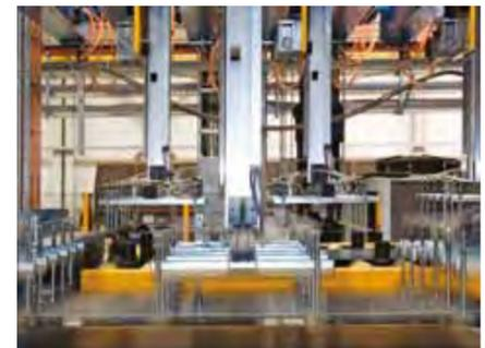
▲ Portal stacker for dimensions of up to 25.4 x 12,000 mm
