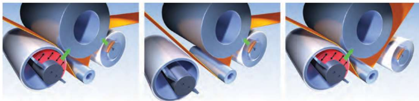
Fig. 2 teXcal trike calender – possible fabric passages
