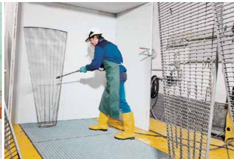
Steam cleaning of segment
