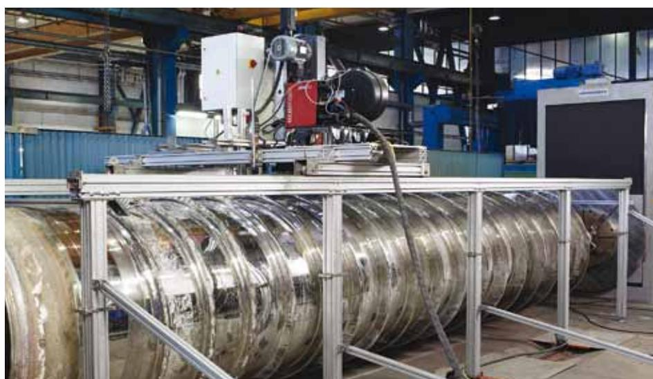
During on-site service a single machining unit is used for welding and grinding. The unit comprises aluminium profiles and a movable tool carriage that runs on rails. It can be set up within a short time and the screw flight repaired rapidly. The technical equipment contains a measuring device
