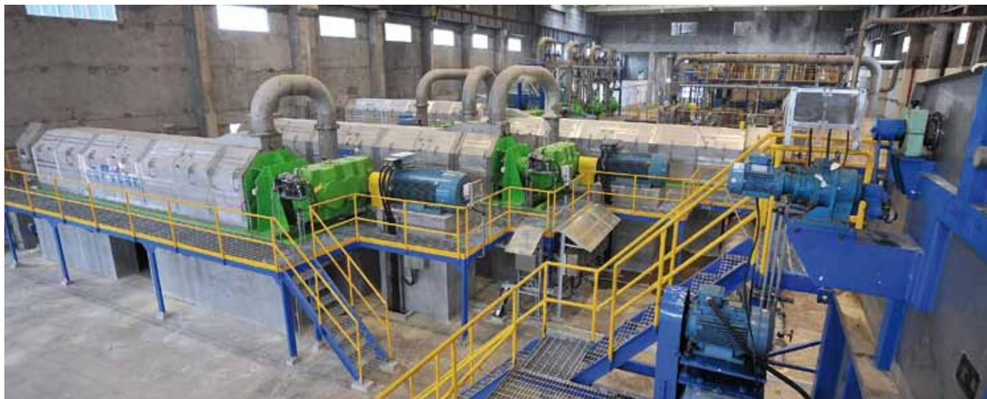
▲ ANDRITZ Screw Presses (SCP1410) as part of a typical four-stage washing system for *P-RC APMP*.
