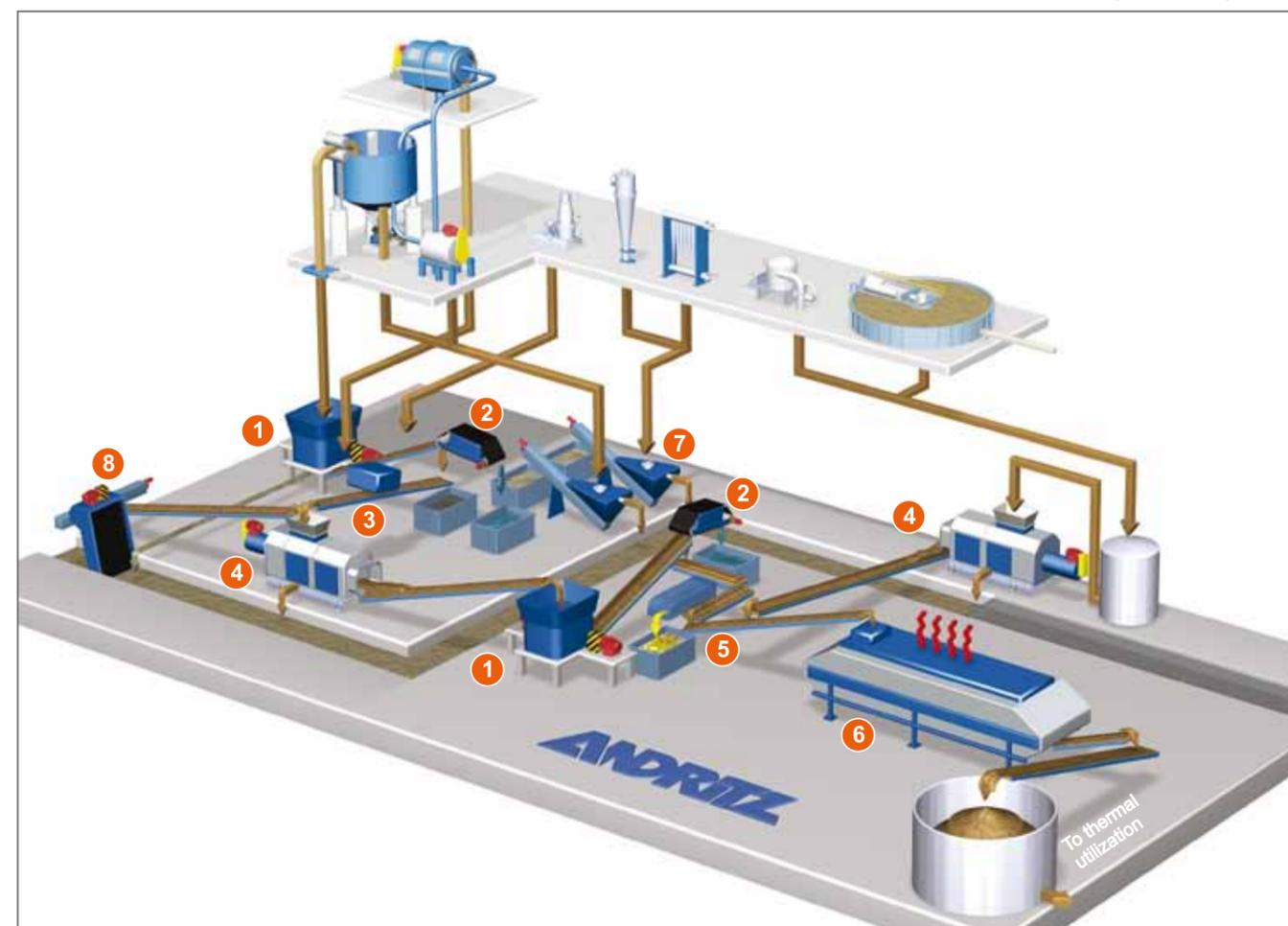
can be detected and classified by means of near infrared technology (NIR). Depending on the end use of the raw material recovered (PVC constitutes a health hazard when incinerated, for example), one or several detected components can be ejected by means of compressed air jets. The separator requires a certain dryness and particle size distribution, and is color-sensitive.
