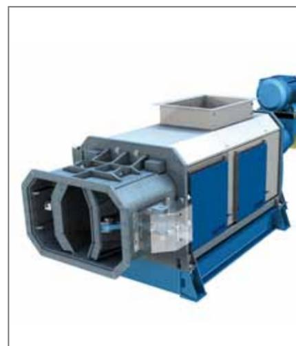
**4 Compacting.** Mechanical dewatering of coarse and fibrous rejects to highest dryness. The reject material fed to the compactor is conveyed by a rotating screw and compressed in a counter-pressure unit by two hydraulically actuated pressure flaps. Wear-resistant, heavy-duty baskets retain the solids, while the water flows through the holes in the baskets and is collected in a filtrate tray. The final dryness depends on the type of reject material and its fiber content.
