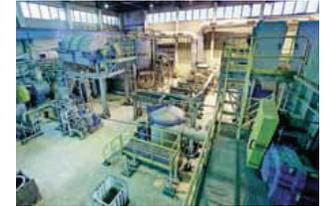
▲ ANDRITZ also delivered a new recycled fiber processing line and machine approach system with a capacity of 800 t/d to bring high-quality stock to PM7's new headbox.
