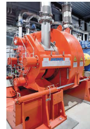
▲ The use of LC refining for the secondary stage or rejects processing contributes to overall energy savings. Shown above is the world's largest LC refiner – the TwinFlo 72.
