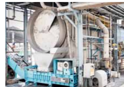
▲ The discharge end of the 300 t/d FibreFlow drum pulper from ANDRITZ.
