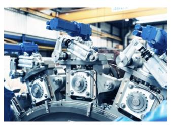
Smart adjustment control of the applicator rolls
