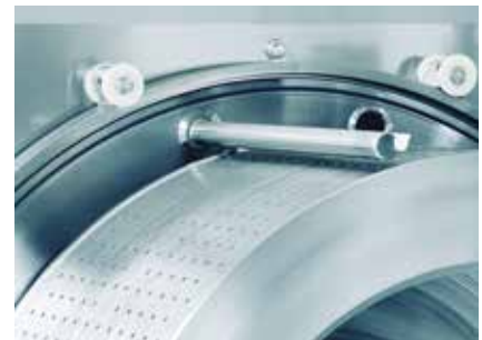
Pneumatic removal of residual heel
