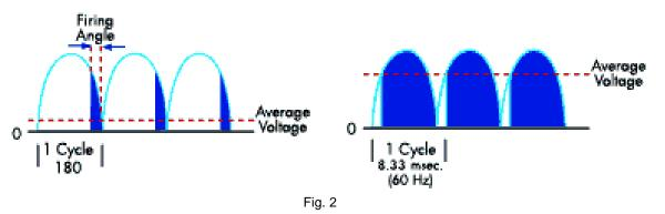
changes in accordance with Ohm's law. The control of current in by this method is termed *"phase control"* as shown in Fig. 2.
