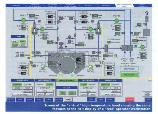
schedule since it is available 24 hours a day. The simulator can be prepared well in advance of the actual equipment startup so that operators are fully trained to take over from the very first moment the machinery is started.
