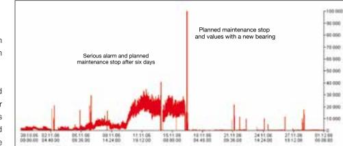
Figure 7: Detailed view of the trend, showing serious fault development in roller bearing as detected by Pulp Dryer ACD
