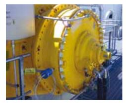
ACU sensors are installed on hydraulic motors for continuous condition diagnostics.
