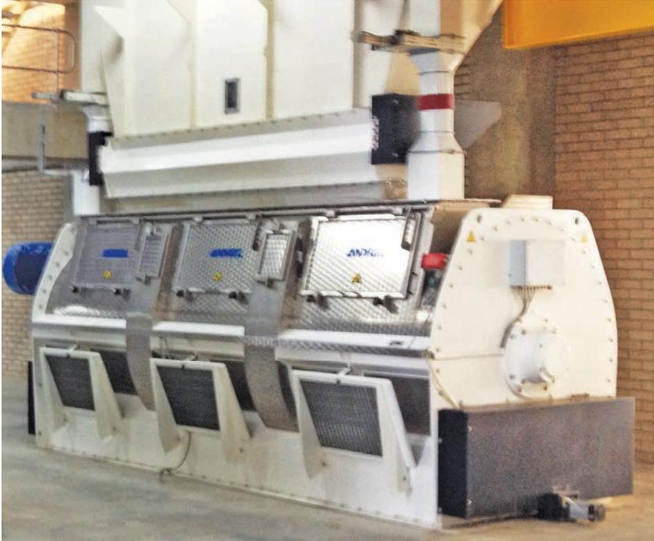
The mixing element consists of a shaft with radially adjustable paddles to ensure maximum mixing accuracy. Scrapers for cleaning of inside gables are also adjustable.
