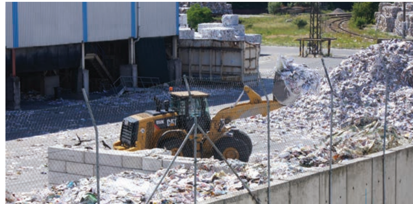
Loose deinking material (illustrated magazines and newsprint) and coated magazines are fed to DIP1.
