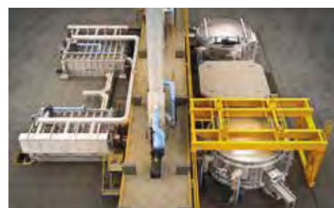
▲ Typical tilting of a holding furnace to ensure uniform flow to the casting machine
