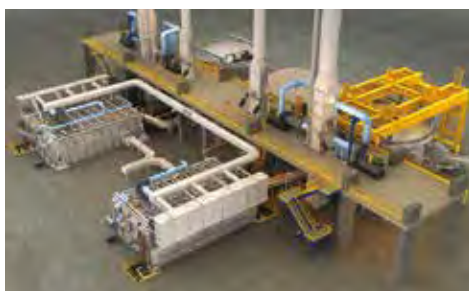
▲ Melter and holder casting cell utilizing 3D design tools help our engineers and your operators to develop, understand and discuss the layout before any soil is broken
