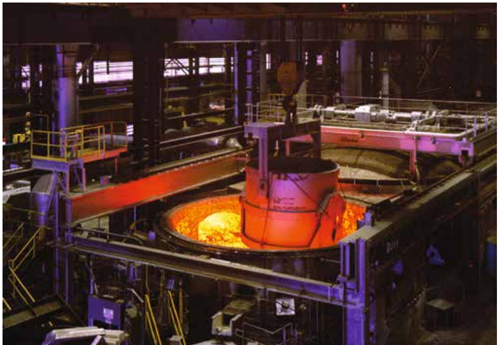
▼ Charging a round top charge furnace
