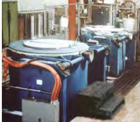
▲ 900 kg (2,000 lbs.) electric tilt crucible furnace
