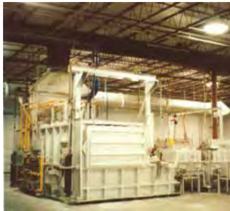
▲ This HI T.E.Q. aluminum melting, transfer, treatment, and holding line includes both gas reverb melting furnaces, and a stack charge furnace for energy efficient melting of returns and scrap.
