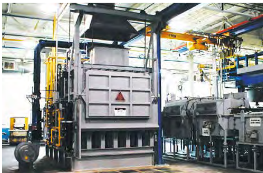
▲ A major manufacturer of marine inboard and outboard engines uses the fully-integrated HiTEQ aluminum melting, metal processing, metal transfer and holding system to supply metal to its lost foam engine block line.
