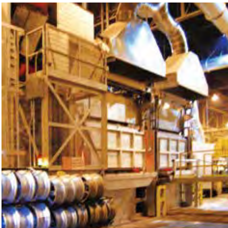
▲ 4,200 kg (9,260 lbs.) per hour stack melter with chip melting option
