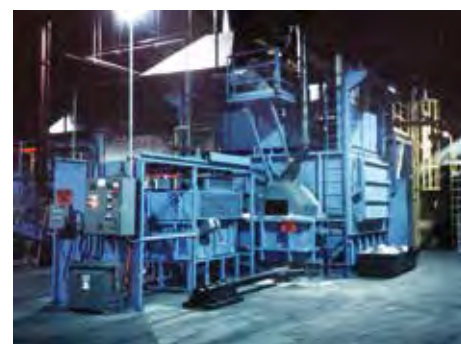
▲ 1,500 kg (4,850 lbs.) per hour chip melting wet bath furnace
