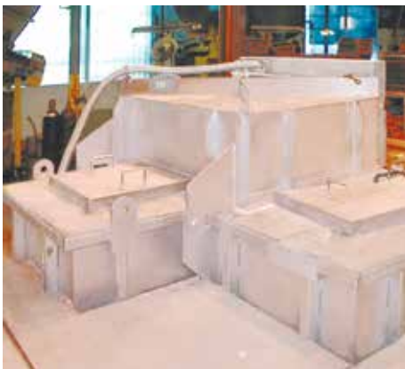
▲ 900 kg (2,000 lbs.) per hour electric radiant resistance melter
