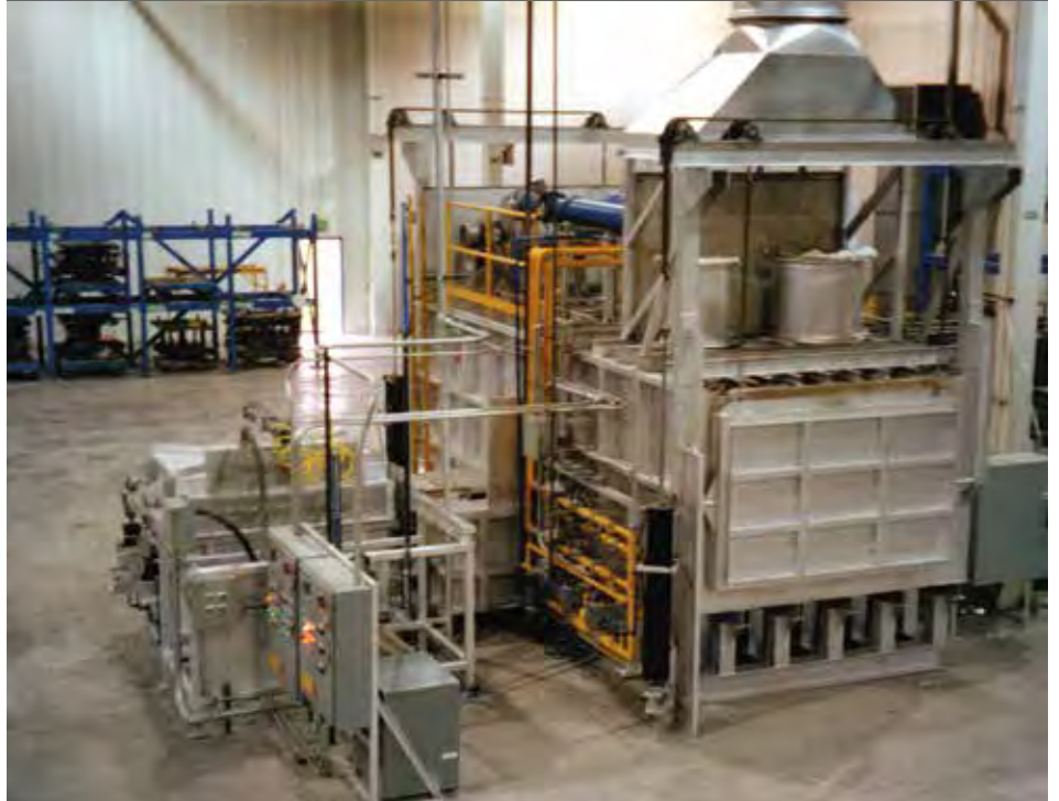
▲ 1,800 kg (3,970 lbs.) per hour dry hearth melter with filtration
