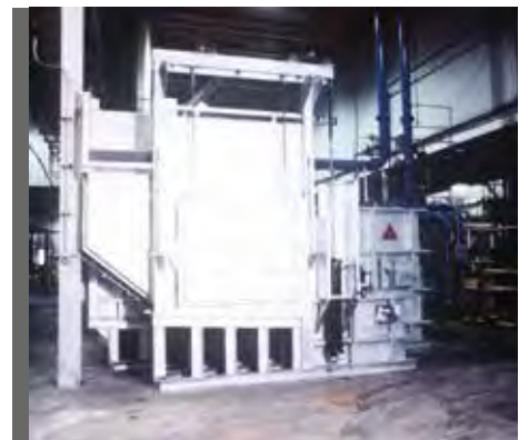
▲ 1,000 kg (2,200 lbs.) per hour dry hearth melter
