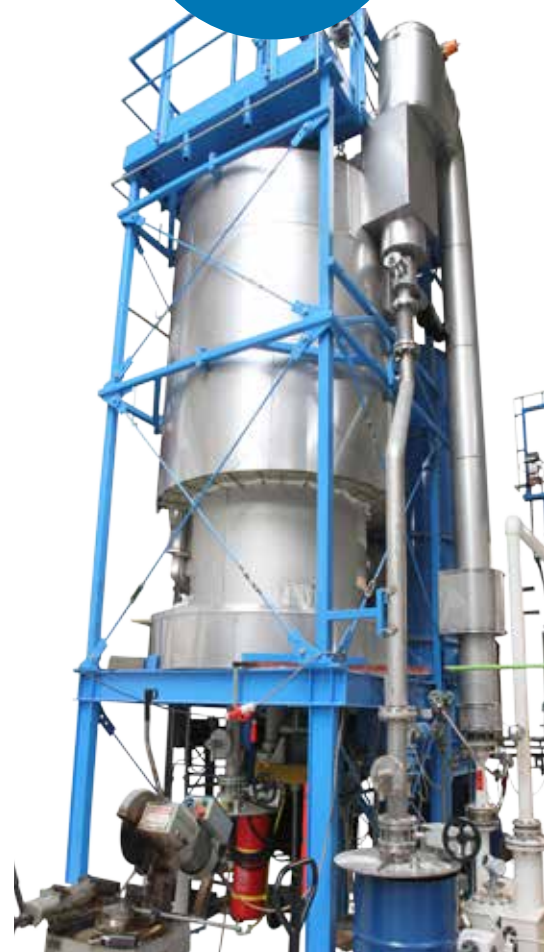
▲ ANDRITZ METALS spray roaster pilot plant
