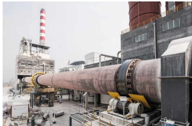
▲ The mill's new white liquor plant from ANDRITZ has capacity to produce 4,800 m 3 /d of white liquor. The LimeKiln shown here can produce 400 t/d of returned lime.
