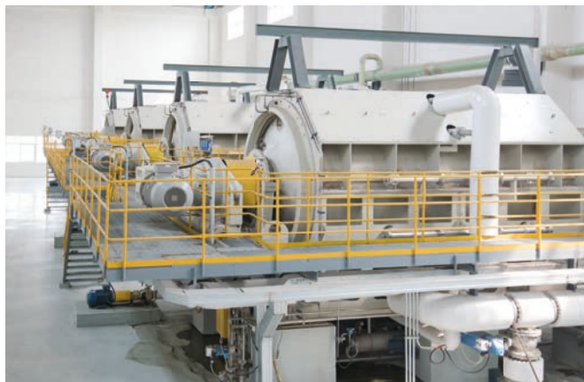
▲ Following the new continuous digester are multi-stage DD Washers for brownstock washing and post-oxygen washing, and a single-stage DD washer after every bleaching stage.
