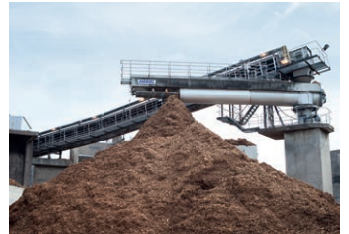
▲ The biomass is a combination of pine, spruce, and birch bark. ANDRITZ delivered a complete biomass handling and conveying system.
