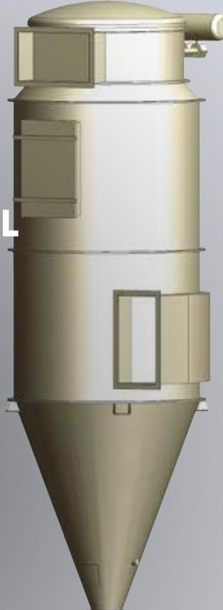
Filter of optimum design for efficient dust separation at low operating cost. Filter type EFF-WB is used for removal of dry dust, especially in large quantities, abrasive dust, or dust with low rates of fall. The product range consists of a fully automatic, continuously operating bag filter cleaned by compressed air and built in series, containing from 10 to
