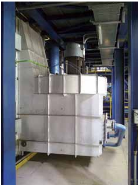
▲ Cooling unit of the Gas Jet Cooling (GJC) section
