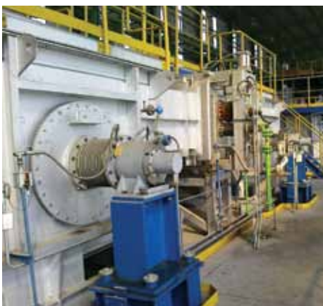
▲ Top transfer preheating and Direct Fire Furnace (DFF)
