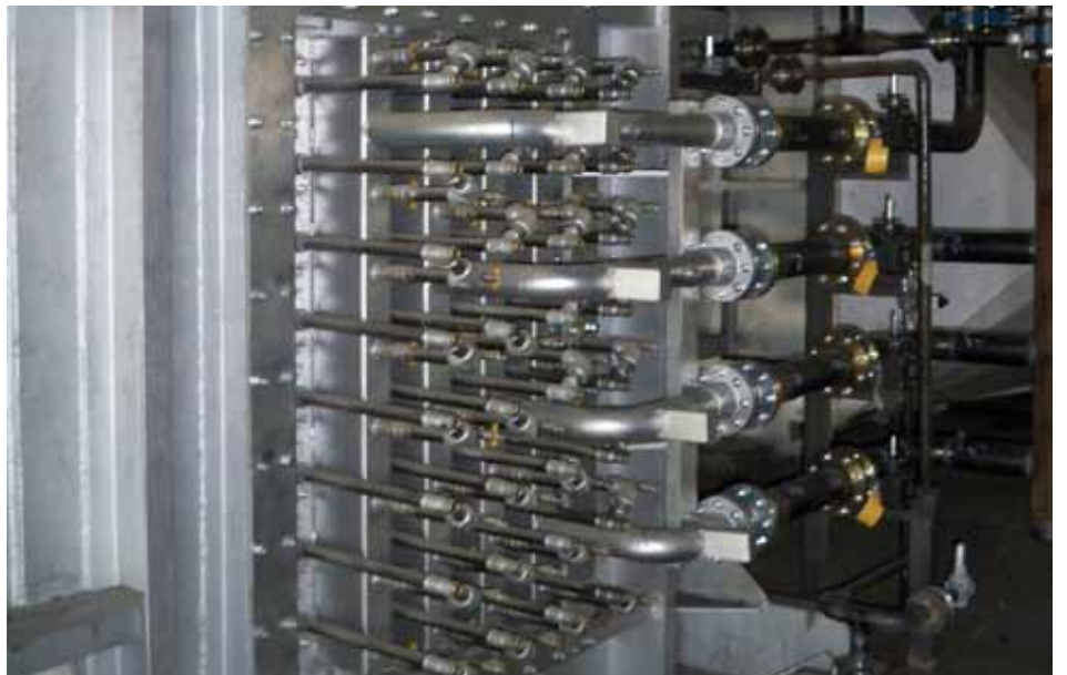
▲ KB burners panel – Direct Fire Furnace (DFF) section
