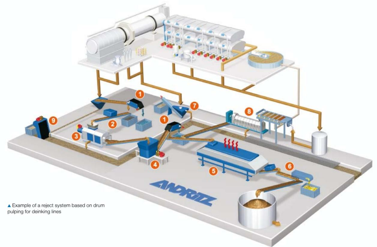
▲ Example of a reject system based on drum pulping for deinking lines
