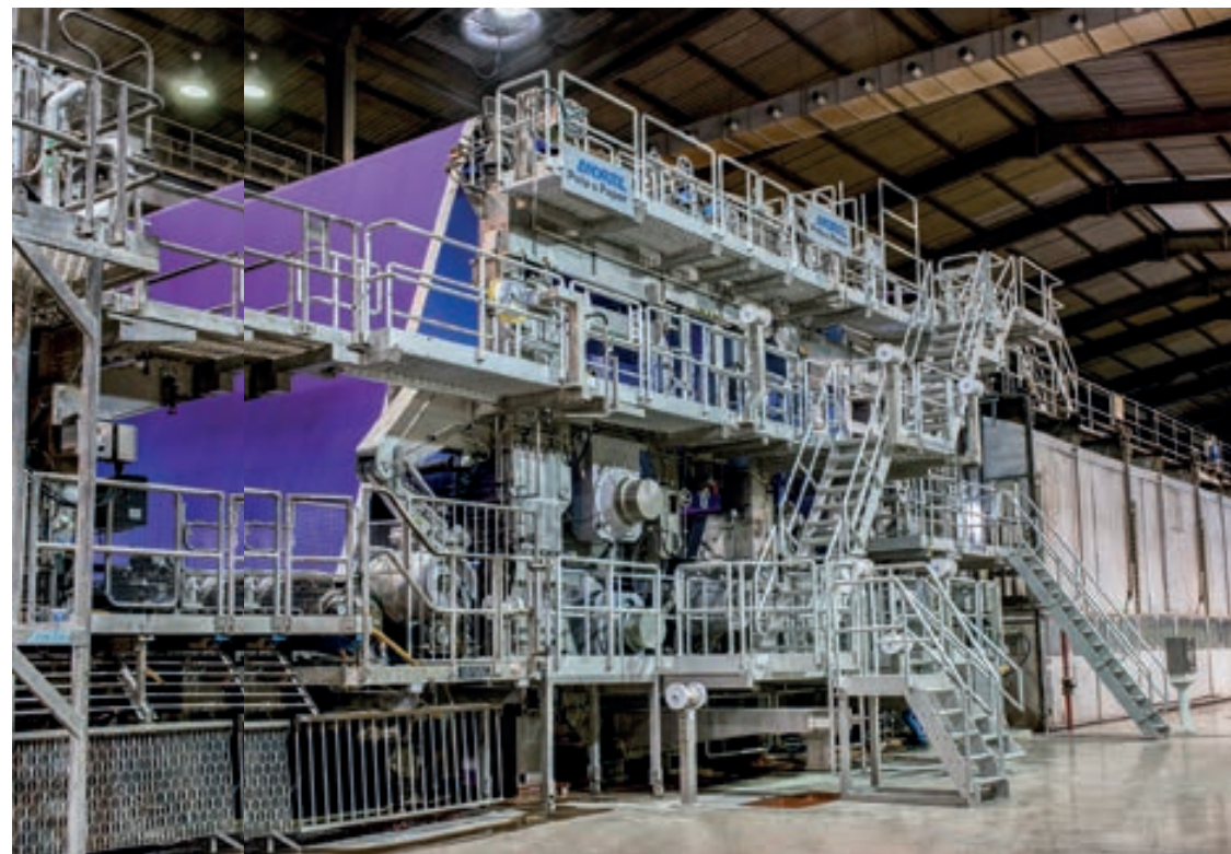
▲ ANDRITZ installed a new press section on Iggesund’s BM2, including a long-nip jumbo press with large-diameter rolls, an energy-efficient PrimePress X shoe press in the second nip, and a smoothing press. The delivery also included ANDRITZ’s state-of-the-art PrimeFeeder vacuum system for ropeless tail threading from the press section to dryer section.
