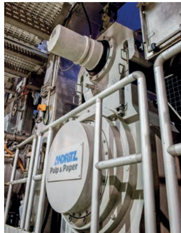
▲ The ANDRITZ PrimePress X shoe press is a very low-maintenance design that gives the Iggesund Workington mill the required bulk and dryness for its premium board products.
