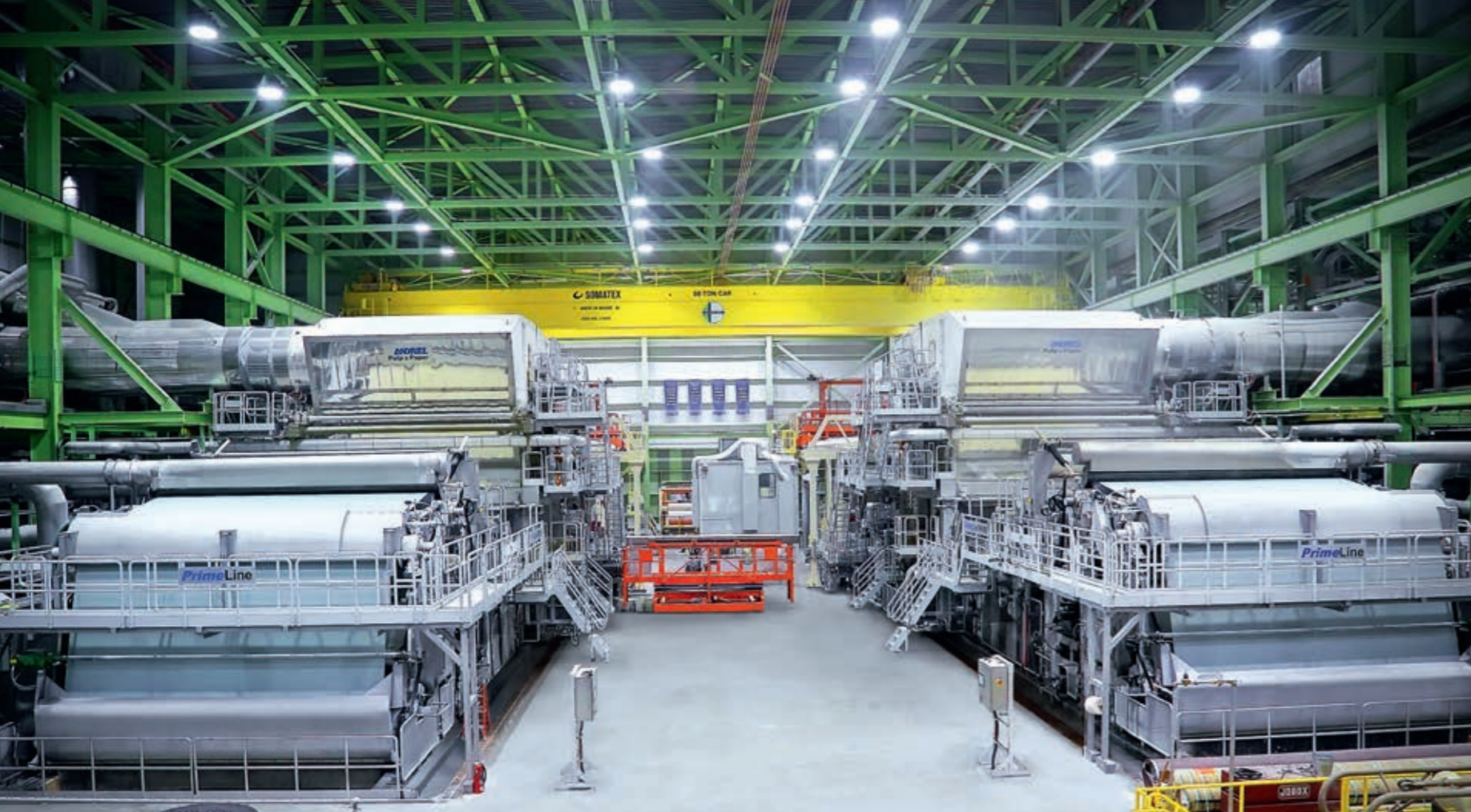
◀ Mirror-image PrimeLine tissue machines. Design speed is 2,000 m/min. Width 5.6 m. Capacity 126,000 t/a combined.
