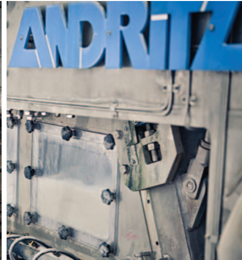
▲ Adding the new PrimeForm HB hybrid former for the filler layer enabled the correct level of dewatering and improved formation.
