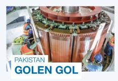
Project update; June 2017; 110 MW; Water & Power development authorities (WAPDA); rotor and stator of unit #1 successfully installed; pre-assembly for unit #2 and #3 ongoing; closing scheduled for end of 2018;
